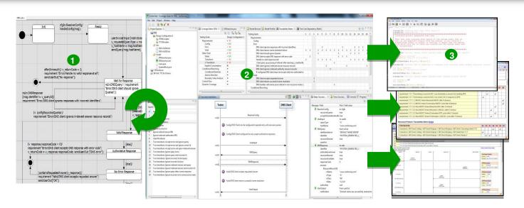
Conformiq Designer's three-step process: 1-model, 2-generate scripts, 3-test execution
