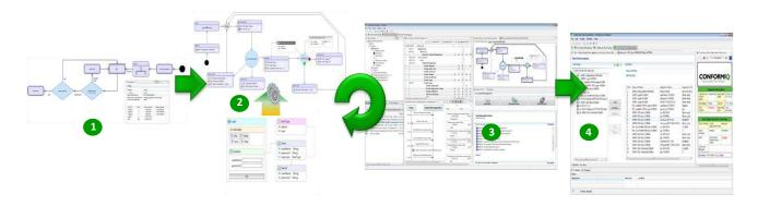
Conformiq Creator version 3 delivers a full agile end2end testing process: 1 - BAs initially model architecture; 2 - testers add interface actions as known; 3 - automatically generate coverage reports, automation scripts and validations; 4 - automated test execution
